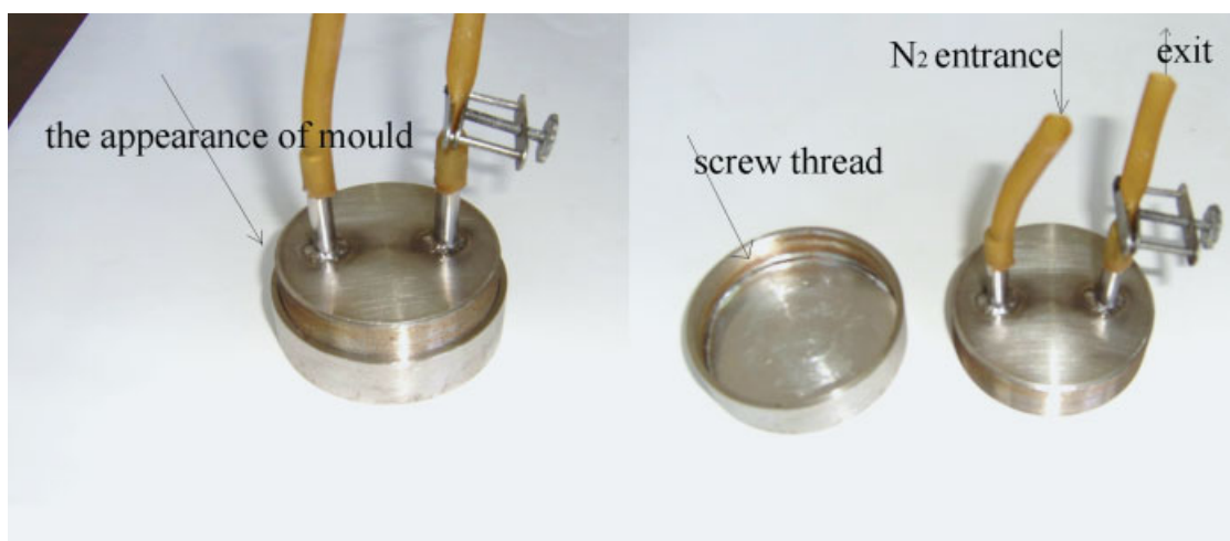
Figure 3 A schematic of the mold used in the thin-layer concentrated emulsion polymerization. [Color figure can be viewed in the online issue, which is available at www.interscience.wiley.com .]
